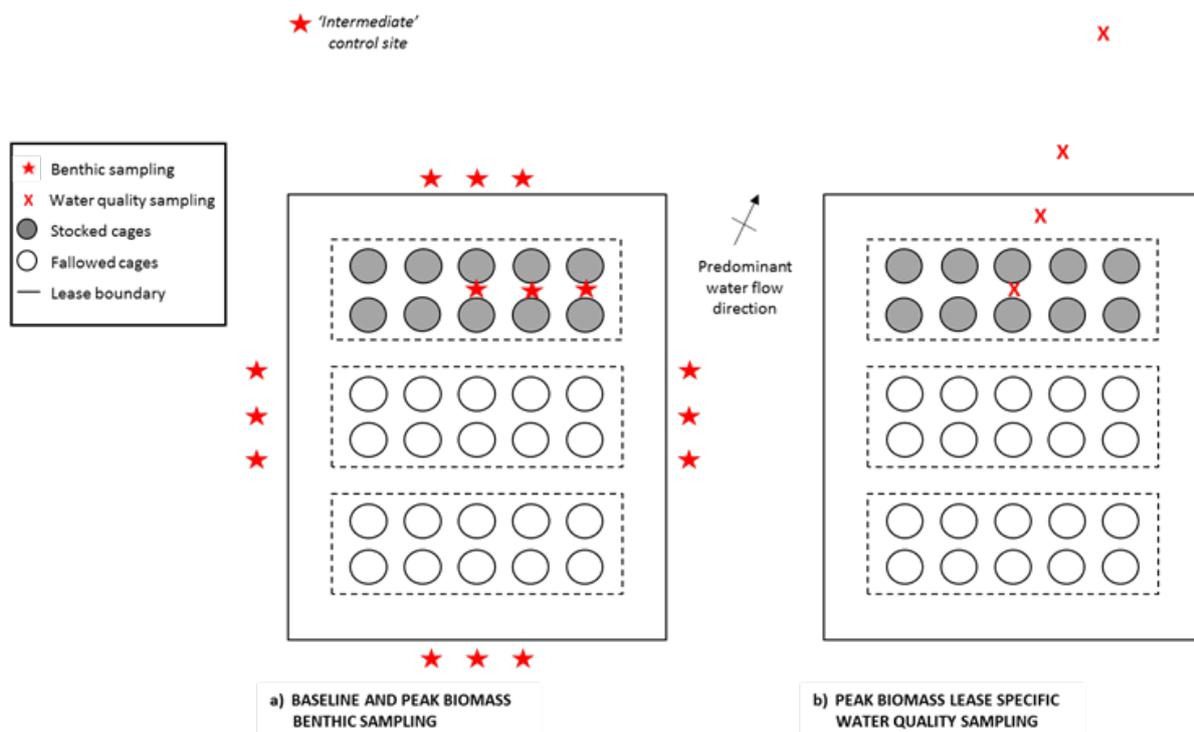
**Figure 2:** Hypothetical finfish marine farming lease area showing location of local/near scale monitoring sites for a) indicative benthic monitoring at baseline and at peak biomass, b) peak biomass/nitrogen output water quality monitoring.
