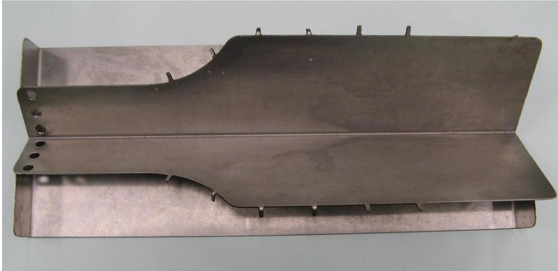
*Fig. 1 Stainless steel cradle for holding large fish for dissection*
