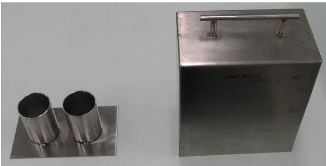
*Fig. 2 Holder for flaming instruments and safety cover*
