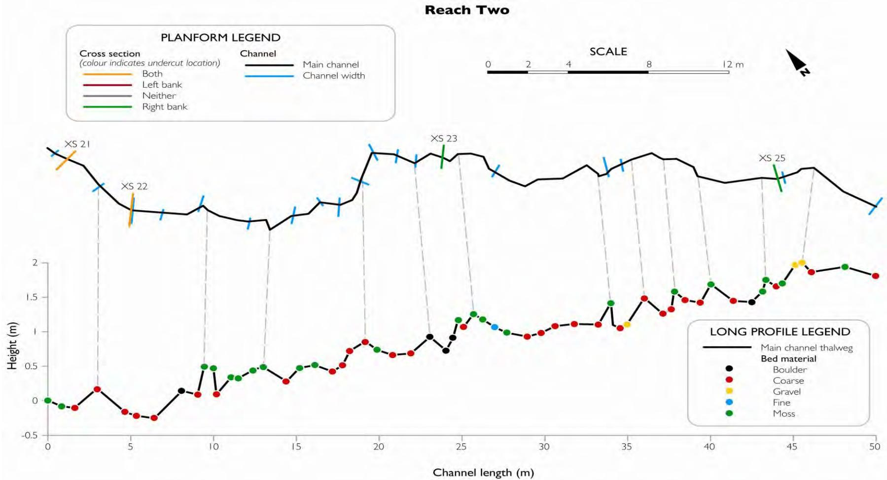
Figure 38. Reach two planform (top) and long profile (in metres from end of reach). Also shown on the planform are channel width at various points, locations of detailed cross sections, and distribution of undercuts. Also shown on the long profile is the bed material on the thalweg. Lines between the diagrams indicate where the control points occur on the planform. Note that scales differ between Figures 37, 38, 39 and 40.
