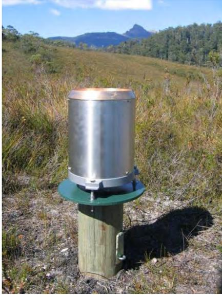
**Figure 4. Tipping bucket rain gauge installed at Galignite Creek.**
