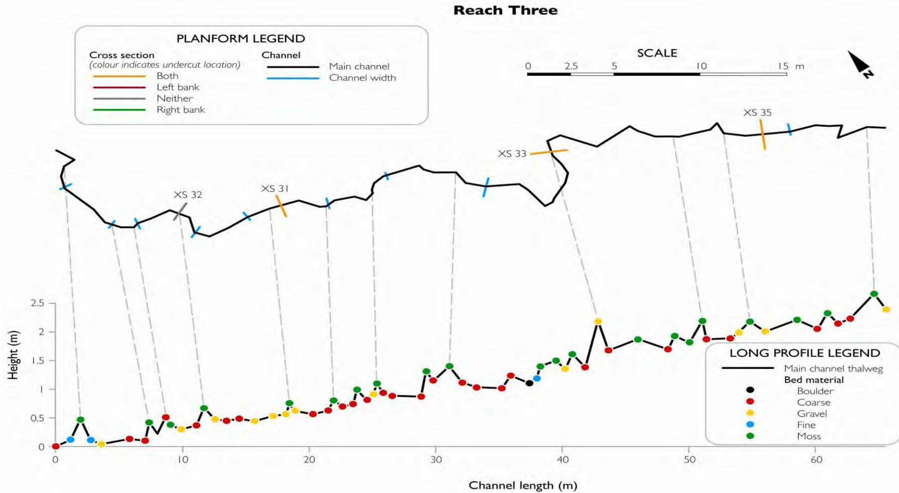
Figure 39. Reach three planform (top) and long profile (in metres from end of reach). Also shown on the planform are channel width at various points, locations of detailed cross sections, and distribution of undercuts. Also shown on the long profile is the bed material on the thalweg. Lines between the diagrams indicate where the control points occur on the planform. Note that scales differ between Figures 37, 38, 39 and 40.
