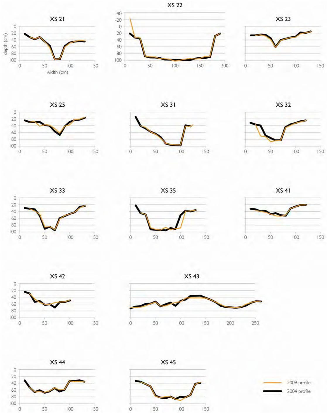
**Figure 42 (continued).** Galignite Creek detailed cross sections from all sites where two measurements are available. Scales are comparable throughout. Undercuts are not depicted. Note that Cross section 43 is of a section where three channels zones were present, but the left most channel was hidden by buttongrass thatch when the cross section was established, and is not completely captured in this data.
