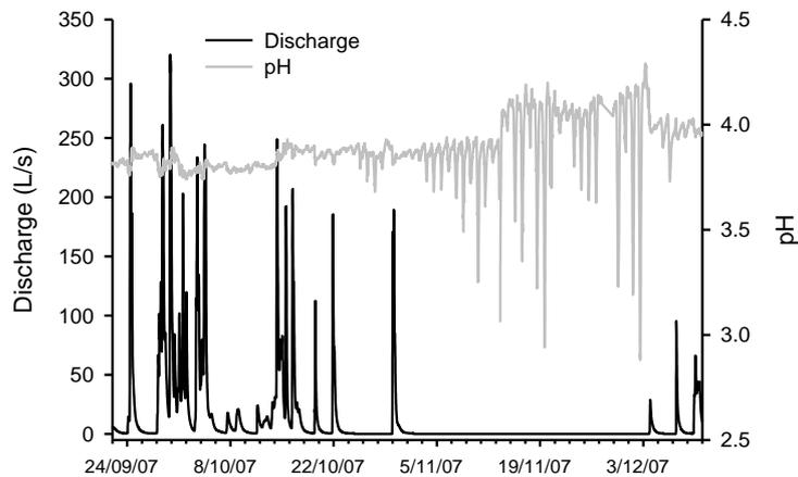
**Figure 29. Galignite Creek discharge and pH between 22/9/2007 and 10/12/2007. Note that pH is generally stable while the stream is flowing, but fluctuates wildly once flow ceases.**
