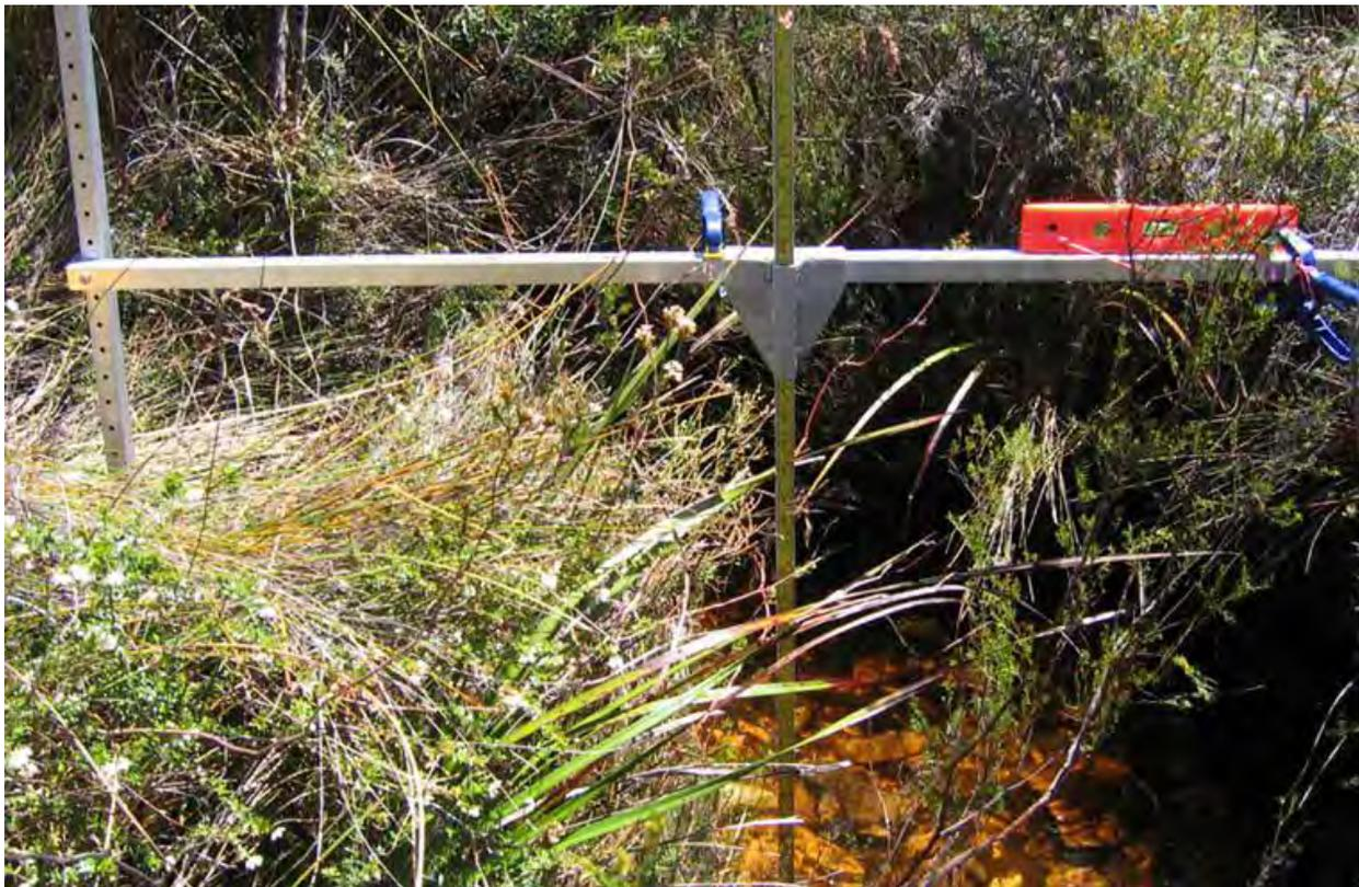
Figure A3-1. Cross section frame set up on Galignite Creek. Flow is away from camera.
