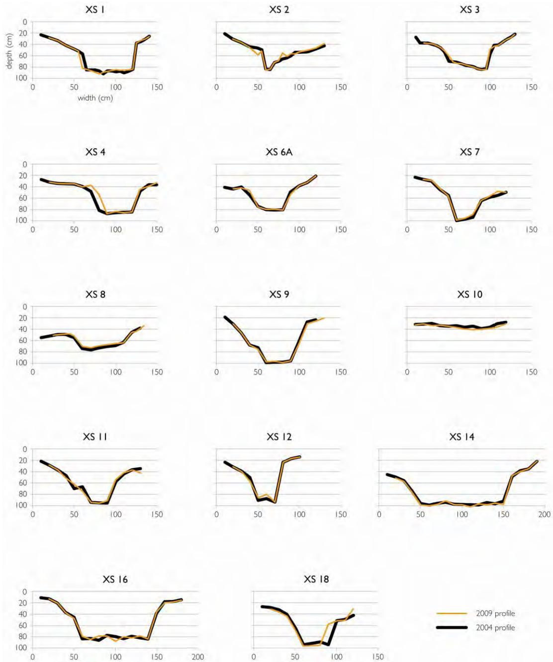
**Figure 41. Galignite Creek detailed cross sections from all sites where two measurements are available. Scales are comparable throughout. Undercuts are not depicted. Note that Cross section 43 is of a section where three channels zones were present, but the left most channel was hidden by buttongrass thatch when the cross section was established, and is not completely captured in this data. (figure continues next page)**
