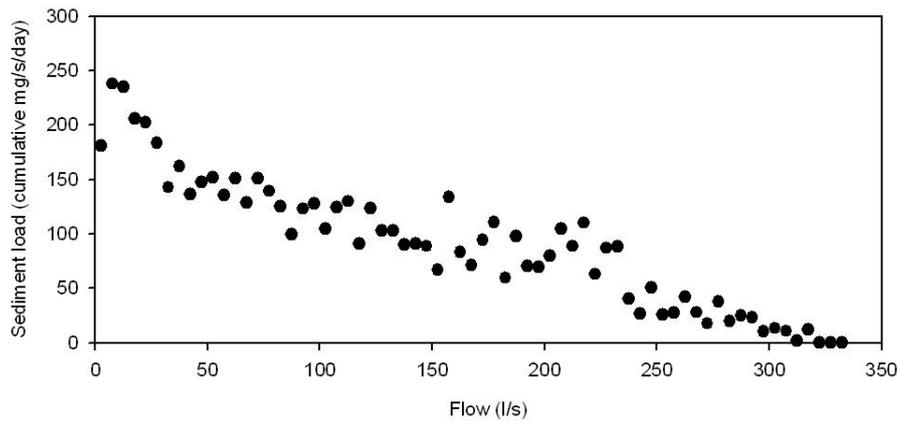
Figure 27. The relationship between estimated average suspended sediment load and flow at the Galignite Creek weir site.
