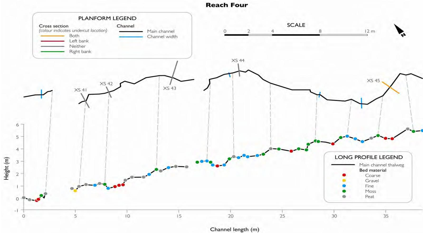
Figure 40 planform (top) and long profile (in metres from end of reach). Gaps in lines reflect the discontinuous nature of the surface channel. Also shown on the planform are channel width at various points, locations of detailed cross sections, and distribution of undercuts. Also shown on the long profile is the bed material on the thalweg. Lines between the diagrams indicate equivalent locations. Note that scales differ between Figures 37, 38, 39 and 40.
