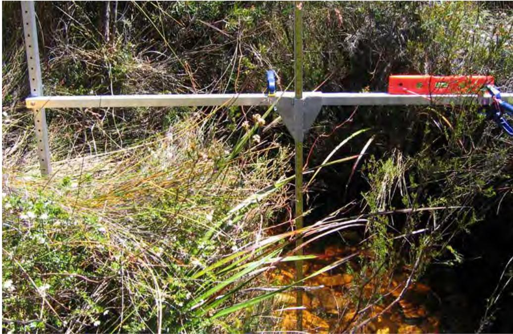
**Figure 6.** The measurement frame set up over a permanent cross section on Reach 1 of Galignite Creek.
