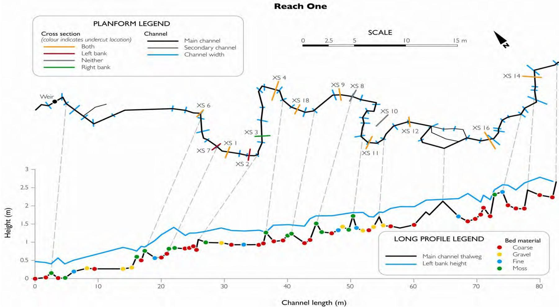
Figure 37. Reach one planform (top) and long profile (in metres from end of reach). Also shown on the planform are channel width at various points, locations of detailed cross sections, and distribution of undercuts. Also shown on the long profile is the height of the left bank and the bed material on the thalweg. Lines between the diagrams indicate where the control points occur on the planform. Note that scales differ between Figures 37, 38, 39 and 40.
