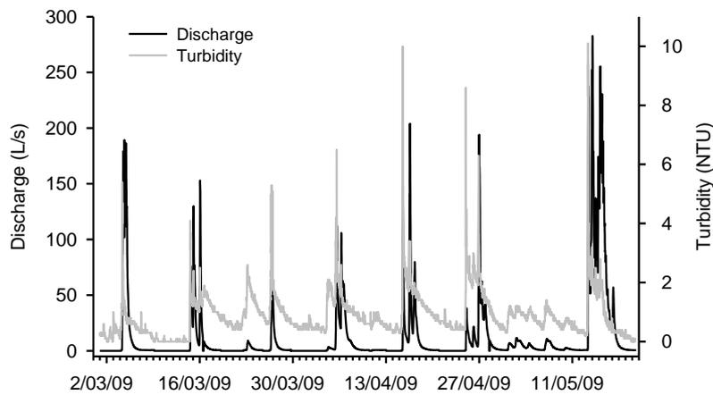
**Figure 32. Gelignite Creek stream discharge (L/s) and turbidity (NTU) over autumn 2009. The relationship between discharge and turbidity of the 26 – 29 March flood is graphed in Figure 33.**
