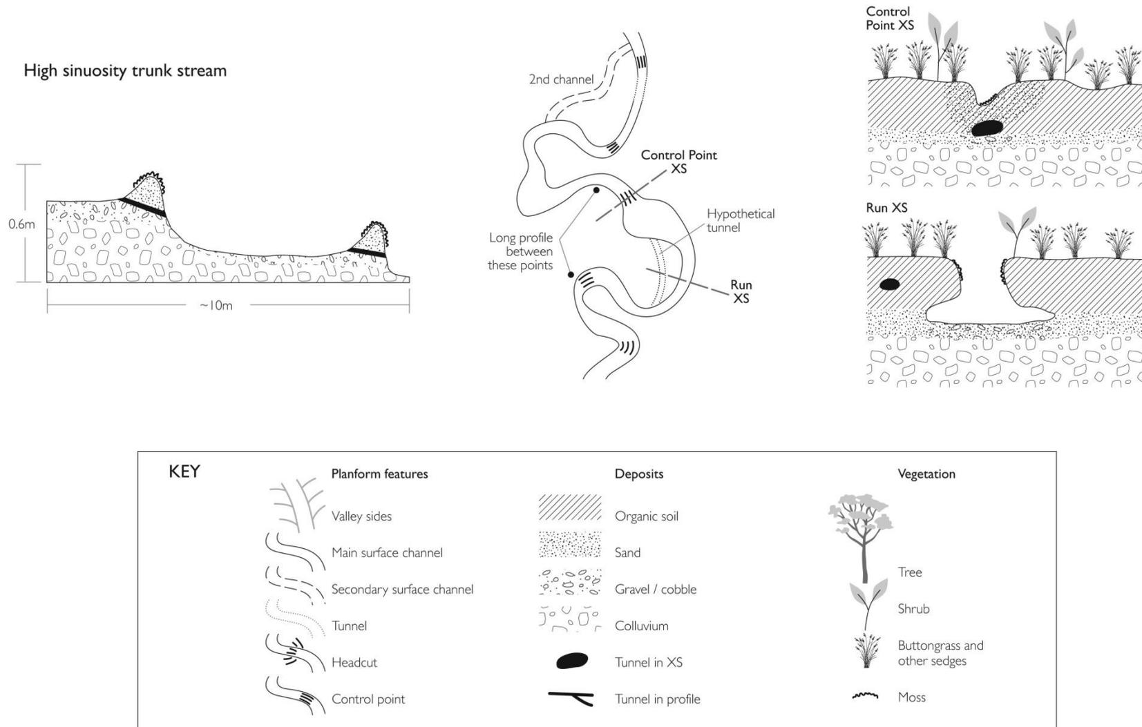
Figure 36. Diagram showing the typical long profile, planform and cross section characteristics of each stream character.
