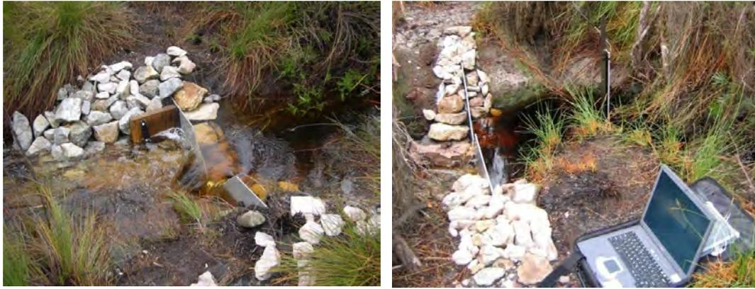
**Figure 5.** Sharp-crested 90° V-notch weir at Galignite Creek (left) and Condominium Creek (right).
