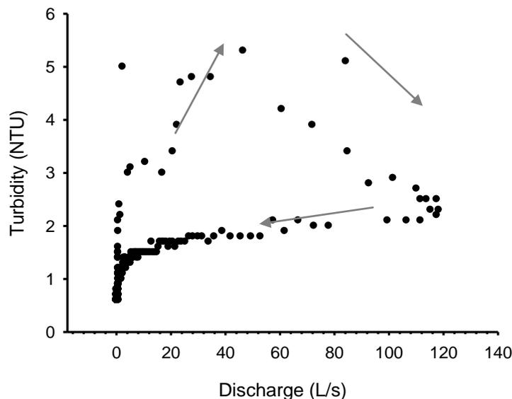
**Figure 33. Turbidity/discharge hysteresis during a storm at Gelignite Creek (26-29/3/2009). Arrows indicate direction of the turbidity/discharge relationship.**
