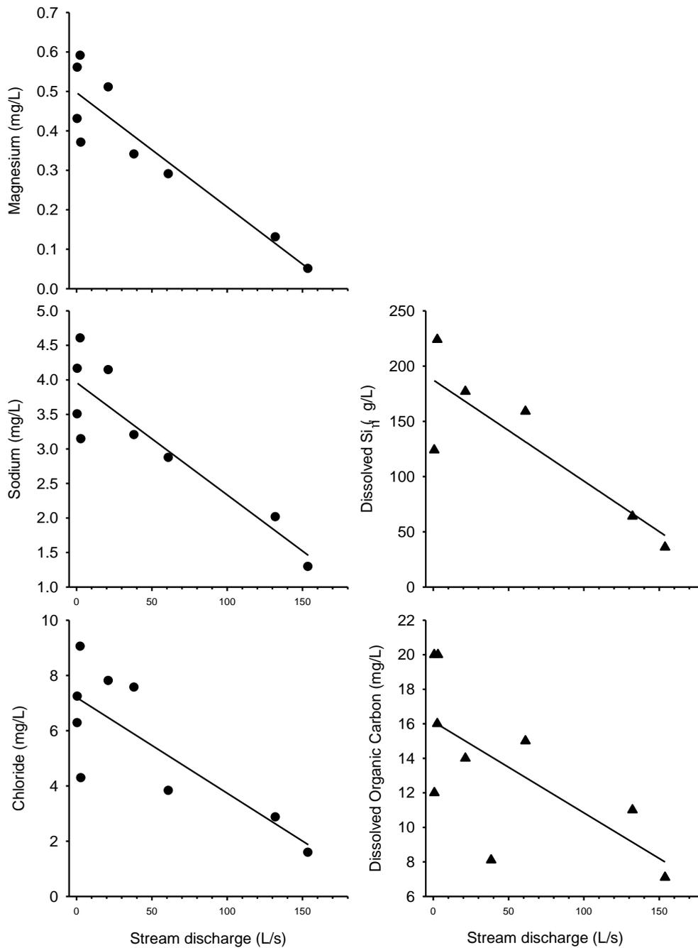
**Figure 34. Relationship between stream discharge and concentrations of dissolved silica ( $\mu\text{g/L}$ ), magnesium ( $\text{mg/L}$ ), and dissolved organic carbon ( $\text{mg/L}$ ). Results from linear regression are shown on the graphs. Analysis of silica, Chloride, sodium and DOC completed using untransformed data, magnesium was log transformed to fulfill assumption of constant variance.**
