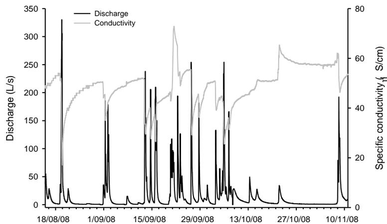
**Figure 30. Galignite Creek stream discharge and specific conductivity between 16/8/2008 and 10/11/2008.**
