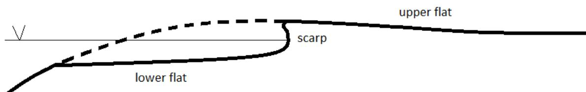
**Figure 4:** A generalised alluvial bank profile showing a near-vertical erosion scarp, typically 30 – 80 cm high, separating two sub-horizontal surfaces.
