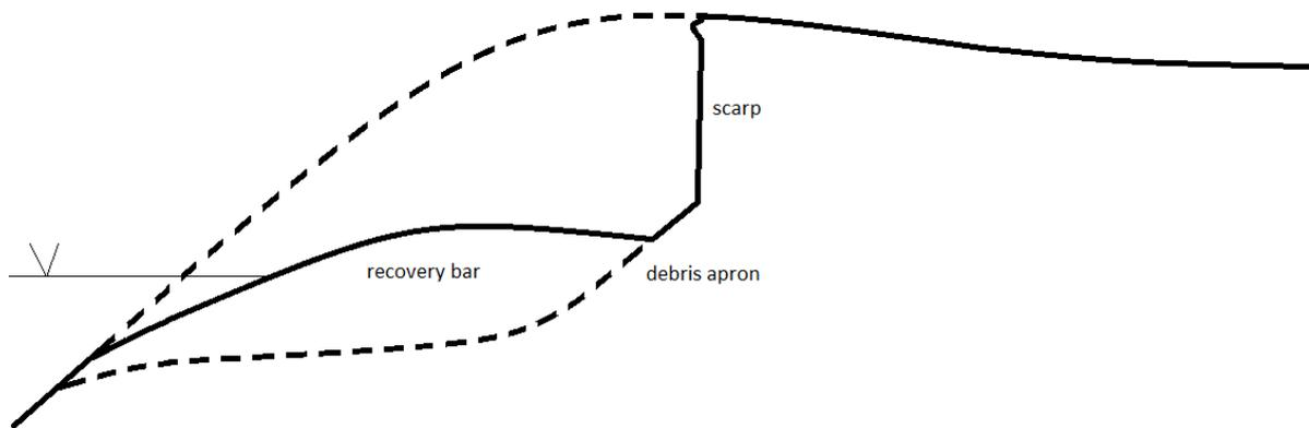
**Figure 6:** Generalised form of levee banks showing upper levee scarp, middle levee debris apron and lower levee recovery bar. The volume removed by erosion during the 1980s is shown between the dashed lines. The top of the scarp is typically 2 – 3.5 m above the normal water level shown.
