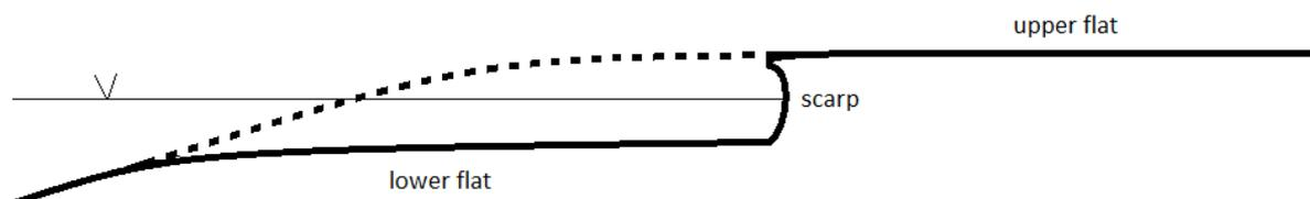
**Figure 2:** A generalised estuarine bank profile showing a near-vertical erosion scarp, typically 30 – 50 cm high, separating two sub-horizontal surfaces. The dashed line shows the pre-erosion profile, as preserved on similar banks in some relatively un-trafficked estuaries elsewhere in southwest Tasmania. The fine line indicates average water level.
