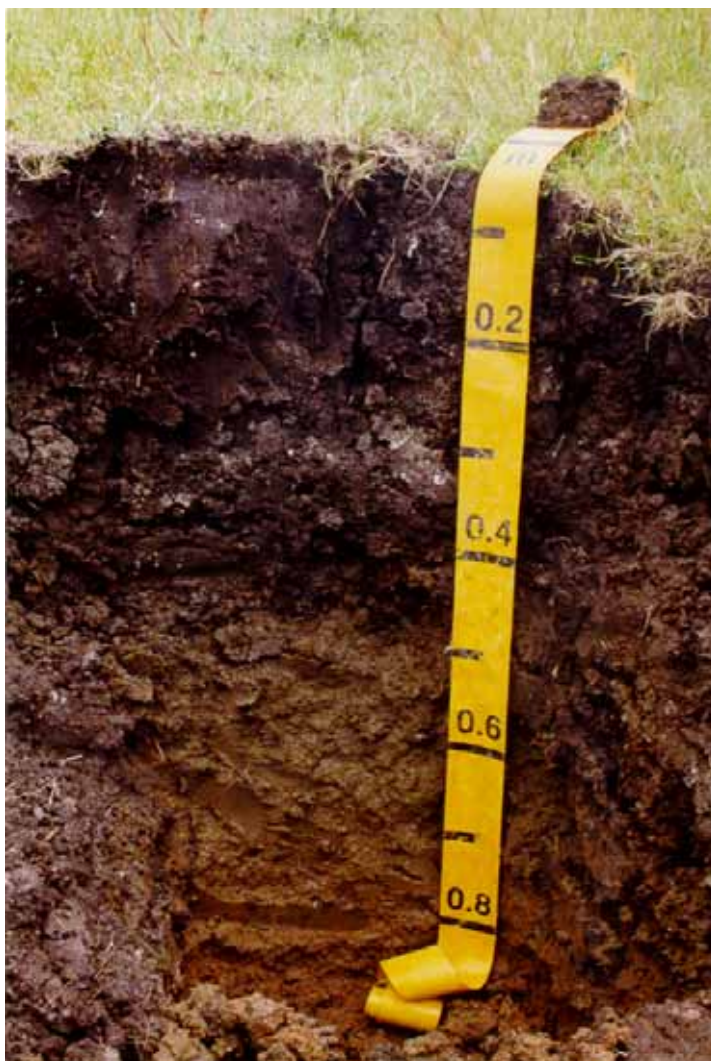
Photo 2. Black Vertosols developed in colluvial dolerite are common on footslope positions. These make reasonable cropping soils where topographic drainage is good (Pitt Water, GR E534400 N5261300).
