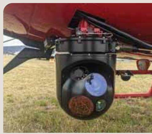
Above, SIG's camera array featuring a precision laser range finder with high resolution visible and thermal infrared sensors.
