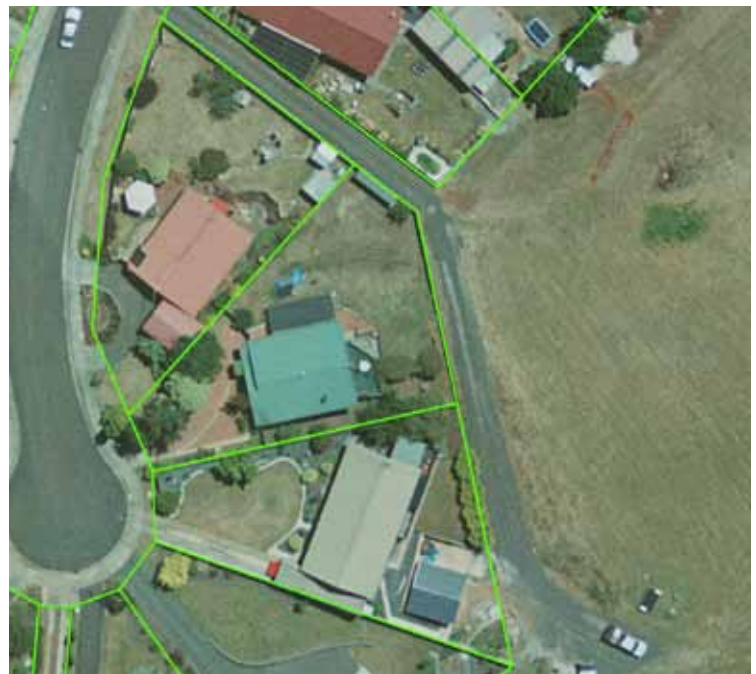
Area of upgraded cadastre showing alignment of other GIS layers.
