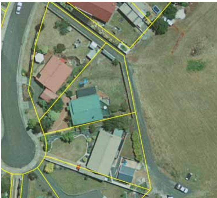
Area of poorly defined cadastre showing misalignment of other GIS layers.
