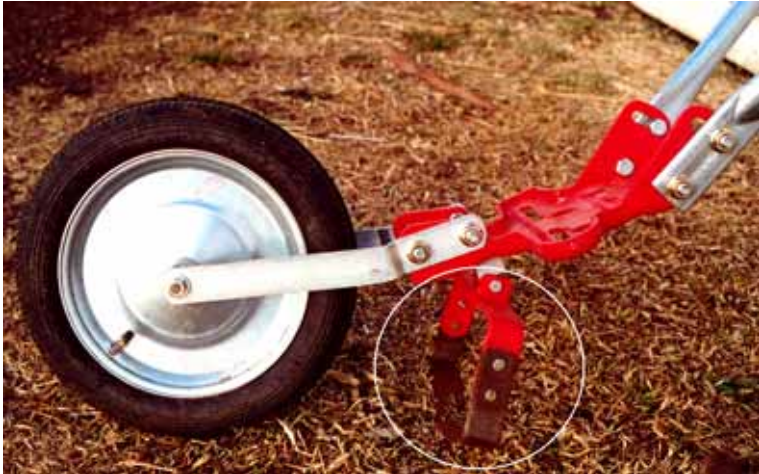
Figure 3.4 Wheel-mounted stirrup hoe used for the hand weeding treatment. The stirrup hoe attachment is circled.
