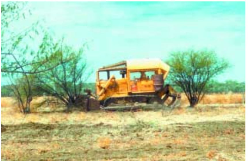
Dozer pushing prickly acacia is especially suited to infestations of medium density over large areas. Photo: Nathan March
