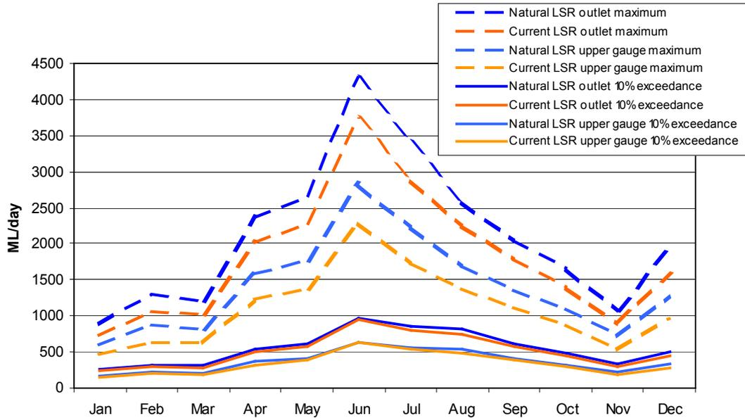
**Figure 6:** Average maximum flows (dashed lines) and 10% exceedance flows (solid lines) for each month in the Little Swanport River at the outlet and the upper gauge, under natural (blue) and current (orange) flow conditions. All flows in ML/day.
