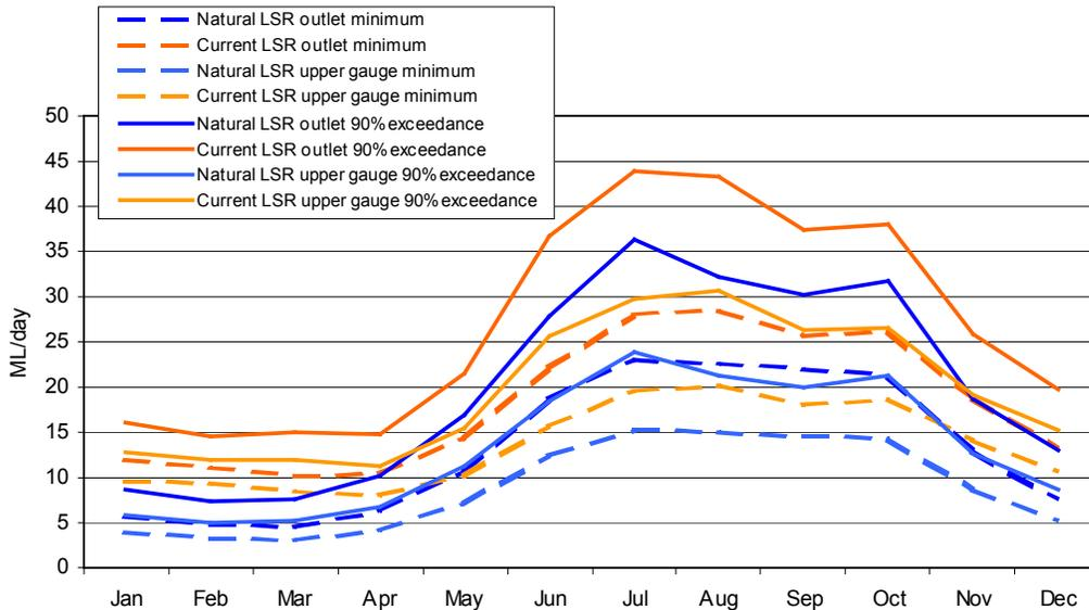
**Figure 7:** Average minimum flows (dashed lines) and 90% exceedance flows (solid lines) for each month in the Little Swanport River at the outlet (blue) and the upper gauge (orange), under natural and current flow conditions. All flows in ML/day.
