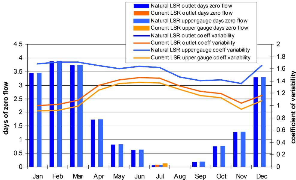
**Figure 8:** Average number of days of zero flow (solid bars) for each month in the Little Swanport River at the outlet and the upper gauge, under natural (in blue) and current (in orange) flow conditions. The solid lines represent the coefficient of variability for each month under natural (blue) and current (orange) flow conditions. The coefficient of variability is the same at the outlet and the upper gauge under natural conditions.
