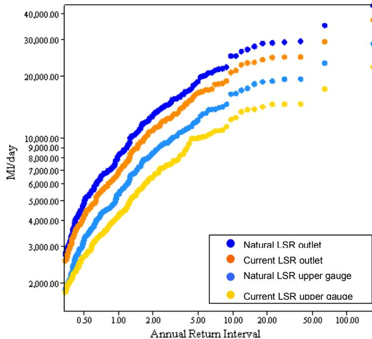
**Figure 9:** Flood frequency analysis of natural (blue) and current (orange) daily flow time series, for the Little Swanport River at the outlet and at the upper gauge. Flood size is in ML/day.
