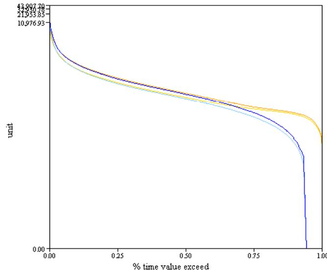
**Figure 4:** Flow duration curves at the Little Swanport outlet under natural (blue) and current (orange) flow conditions, and also at the Little Swanport upper gauge under natural (light blue) and current (yellow) flow conditions.
