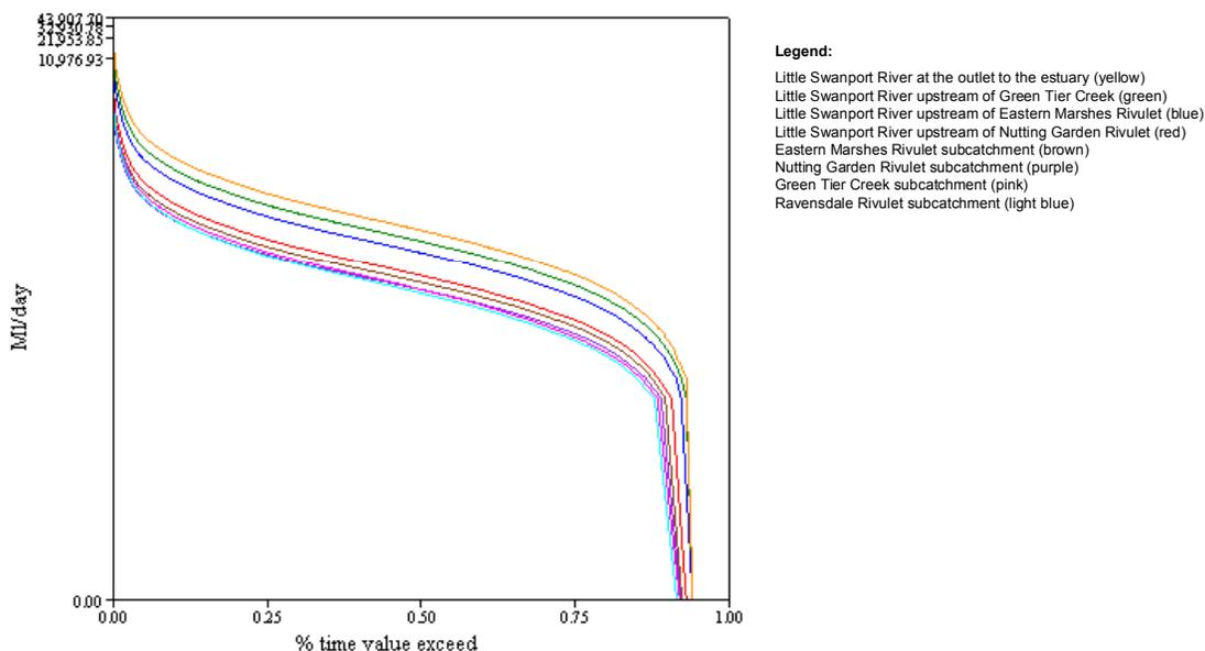
**Figure 3:** Flow duration curves showing the relationship between streamflow (in ML/day) and the percentage of time it is exceeded under natural flow conditions, from selected locations throughout the Little Swanport catchment (see text for interpretation):
