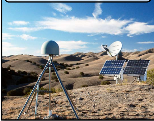
Figure 3 A permanent GPS receiver (left) installed in the United States.
